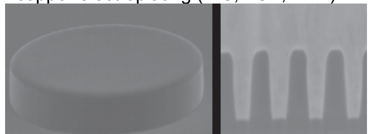
High speed Cu electroplating of flat and uniform patterns (Bumps, Damascene)
