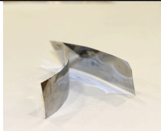
Controlled expansion alloy films for shadow masks, bimetallic actuators
