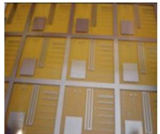
Selective electroless metal plating over a catalytic photoresist on glass substrate
