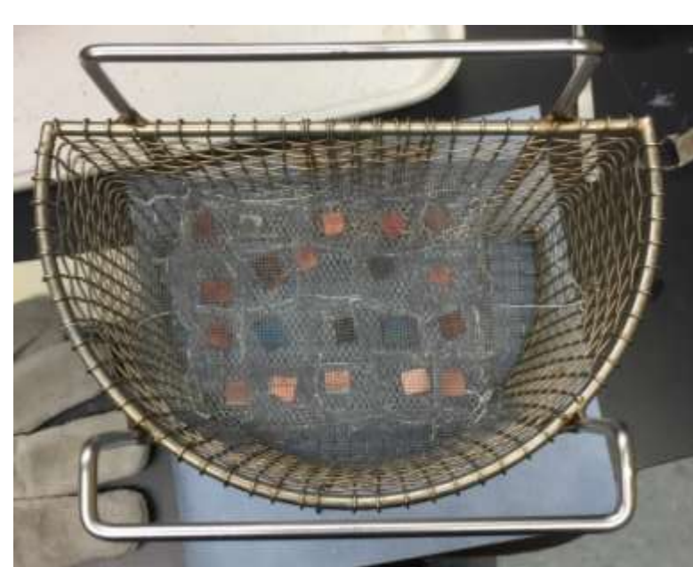
Fig. 5 Thermal Shock Testing Set Up (a) Test Fixture (b) Inside Thermal Shock Chamber
