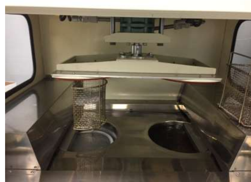
Fig. 5 Thermal Shock Testing Set Up (a) Test Fixture (b) Inside Thermal Shock Chamber
