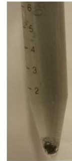
Stabilizer free solution After Ni deposition
