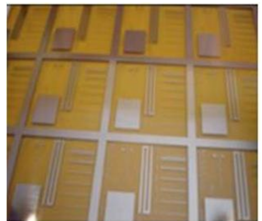
Selective electroless metal plating over a catalytic photoresist on glass substrate
